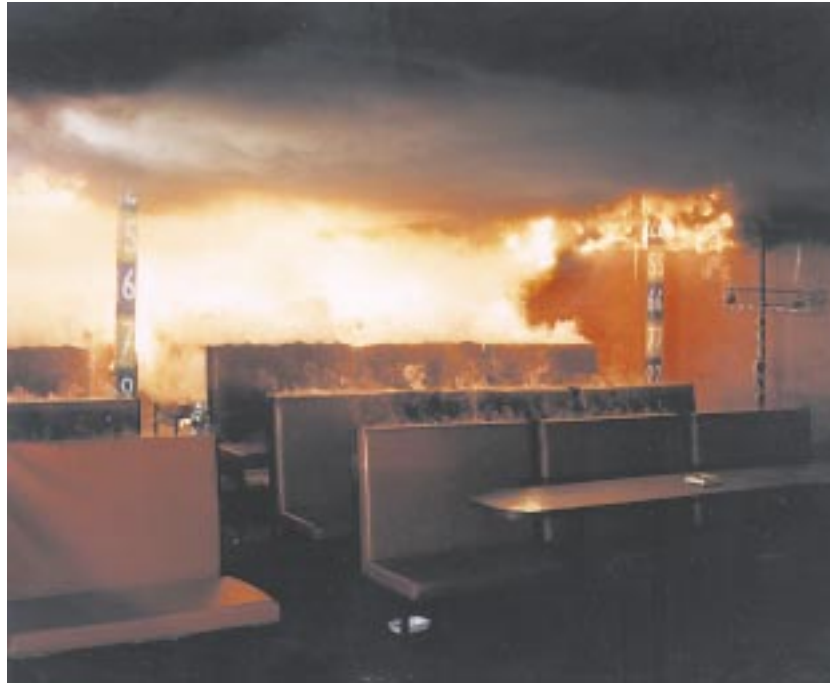
Figure 1. Full-scale reconstruction of the events leading to the fire at the Stardust Discotheque. (Photograph: courtesy of Building Research Establishment Ltd.)
