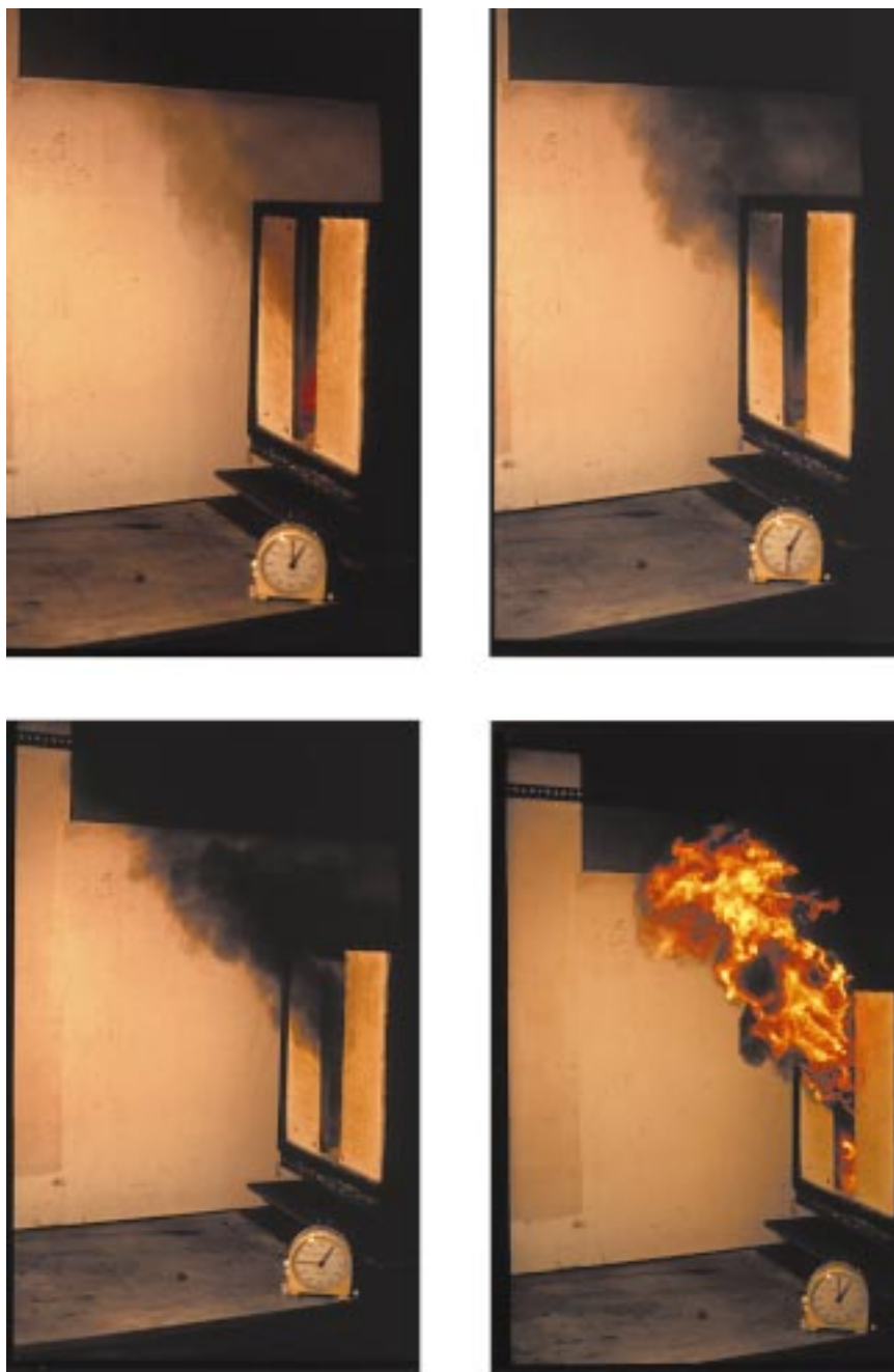
Figure 2. Demonstration of flashover in a small-scale compartment (internal dimensions, 0.4\text{ m} \times 0.4\text{ m} \times 0.4\text{ m} ), with 120 g polypropylene in the form of 6 mm thick strips ( 100\text{ mm} \times 10\text{ mm} ) contained in a lightweight mild steel tray ( 0.2\text{ m} \times 0.3\text{ m} , by 0.01\text{ m} deep). The ventilation opening was 0.1\text{ m} wide, 0.4\text{ m} high. Ignition was achieved by igniting 100 ml of methyl alcohol in the tray: (a) 4 min 00 s; (b) 4:30; (c) 4:45; (d) 5:00. Thereafter, the polypropylene burned out within 45 s.
